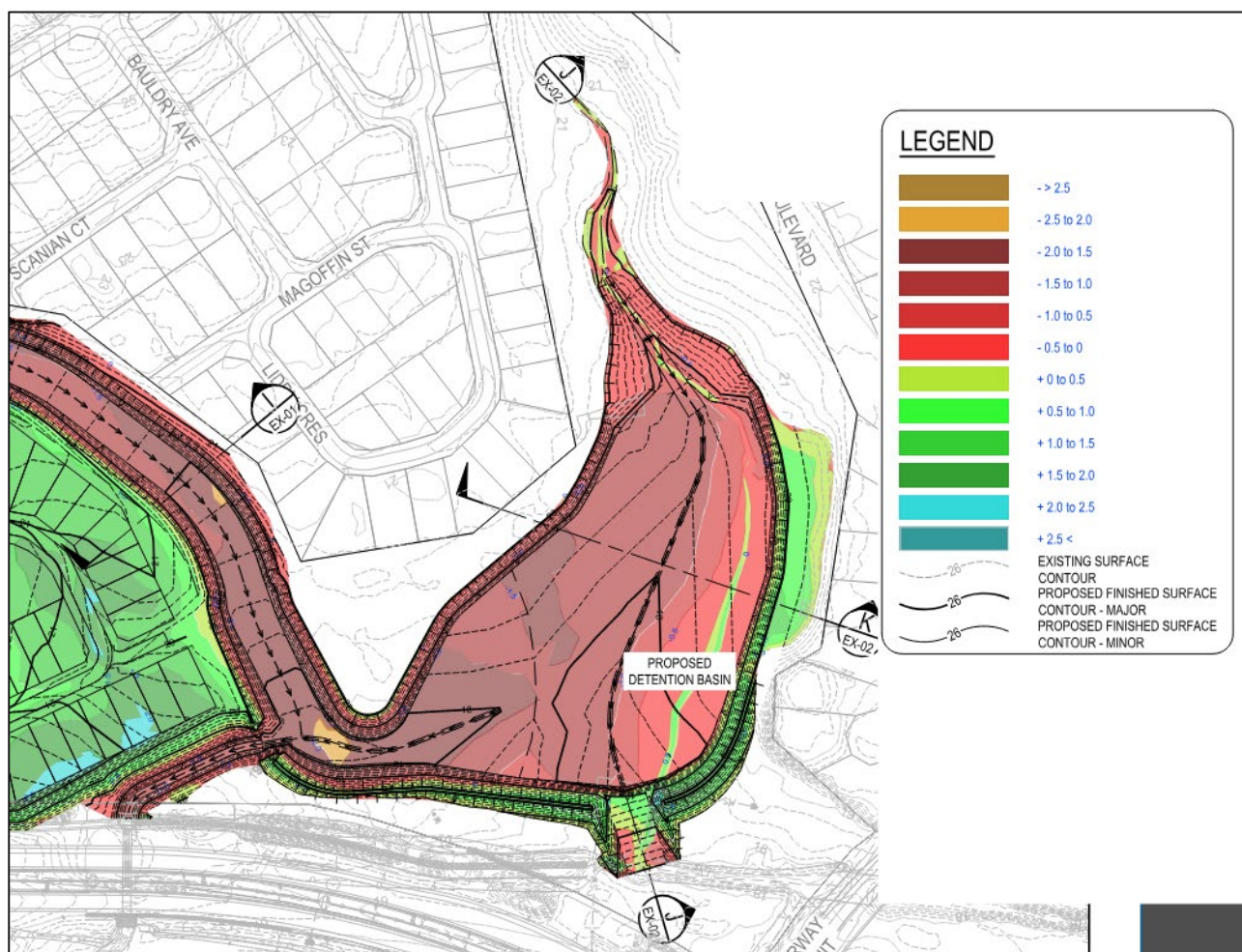
Figure 19: Proposed Detention Basin Earthworks
