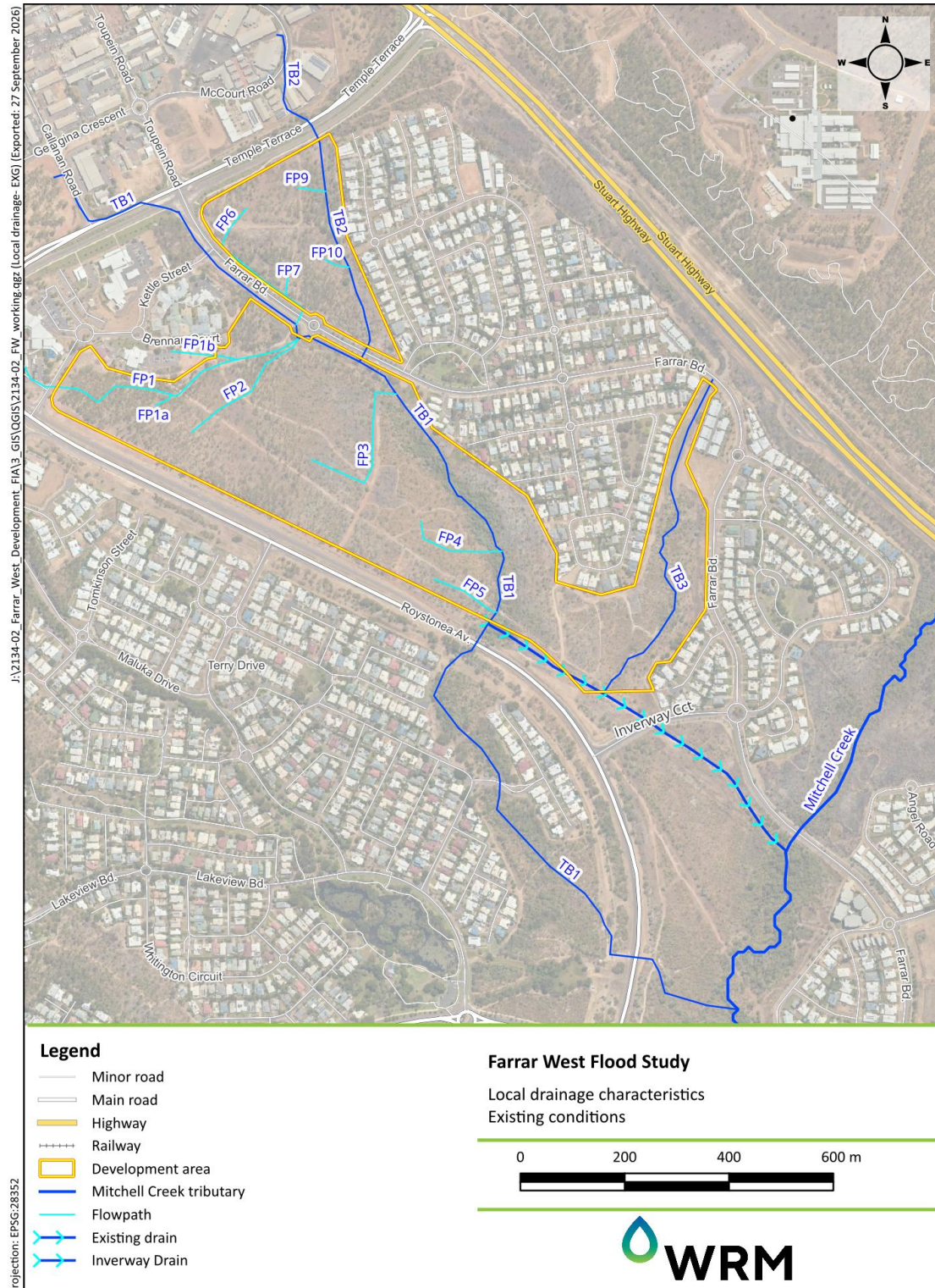
Figure 2.2 Local drainage characteristic – Existing conditions
