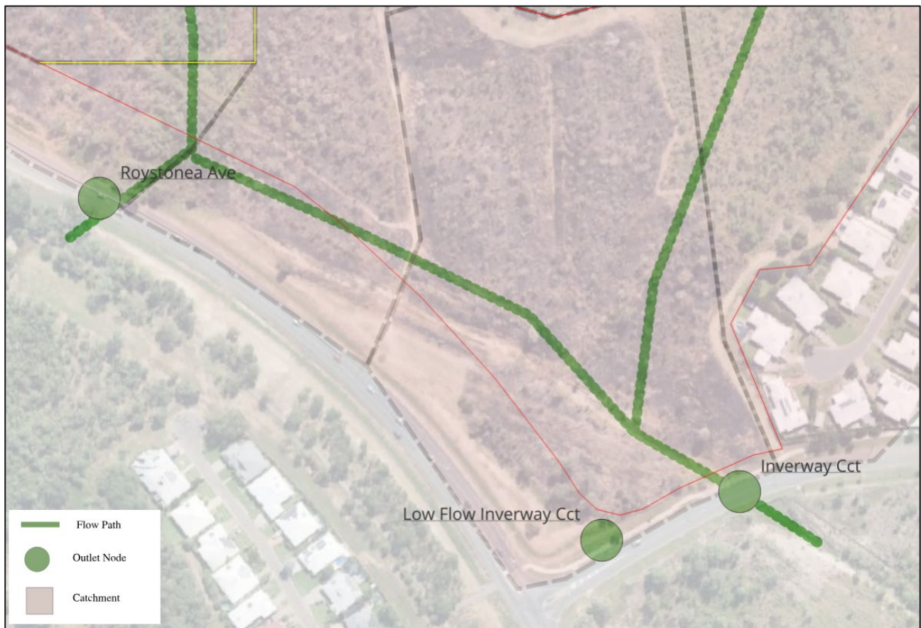
Figure 21: Site Discharge Points
