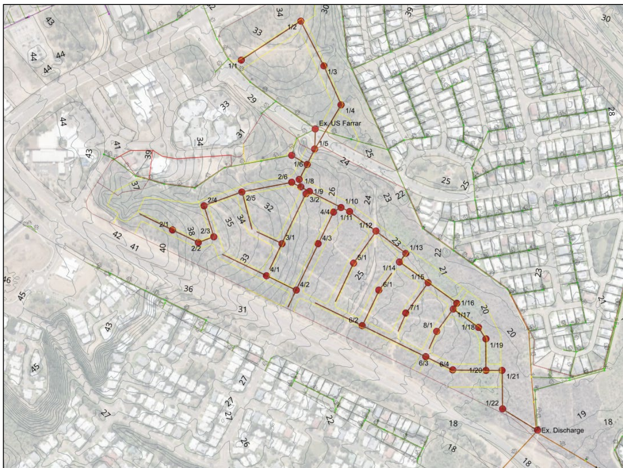
Figure 13: Preliminary Sewer Layout
