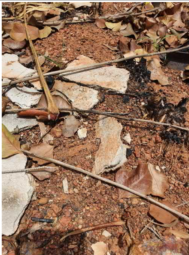
Photograph 05: Suspected ACM within stockpiles on the northern boundary of Lot 5.
