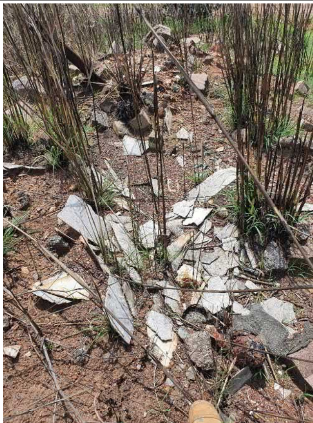
Photograph 06: ACM material, confirmed with laboratory analysis, Observation location 33.
