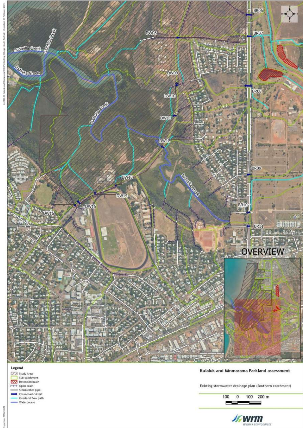
Figure 12.3 – Existing Drainage Catchments – South
