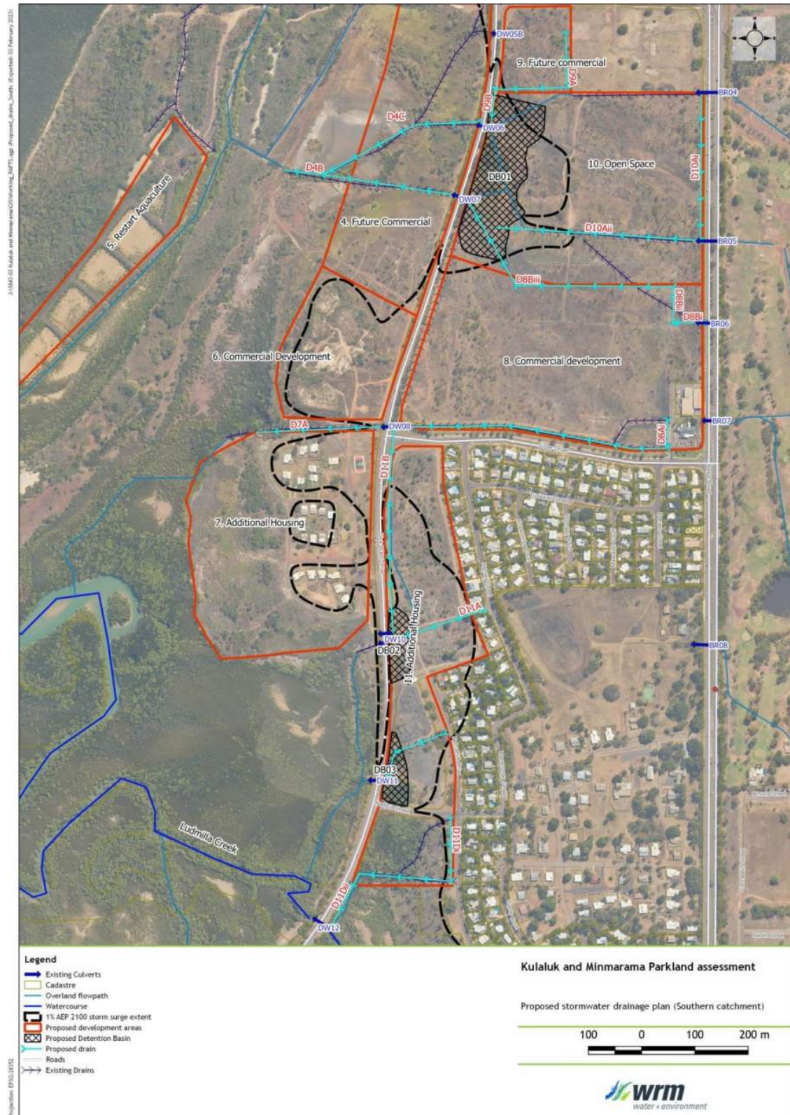
Figure 15.4 – Stormwater Drainage Plan – South
