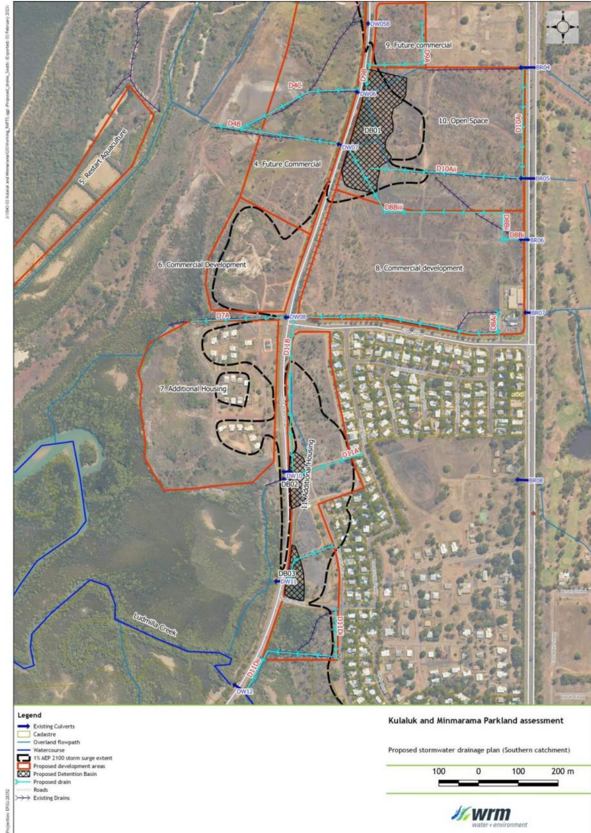
Figure 12.5 – Proposed Stormwater Drainage
