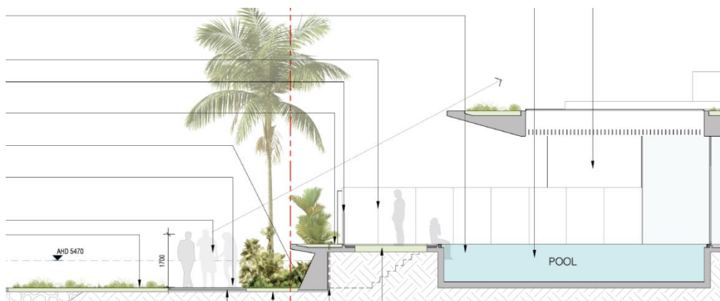
Image 10: Level difference between foreshore villas and public foreshore pathway (image source: Architectural Plan – Foreshore Interface)
