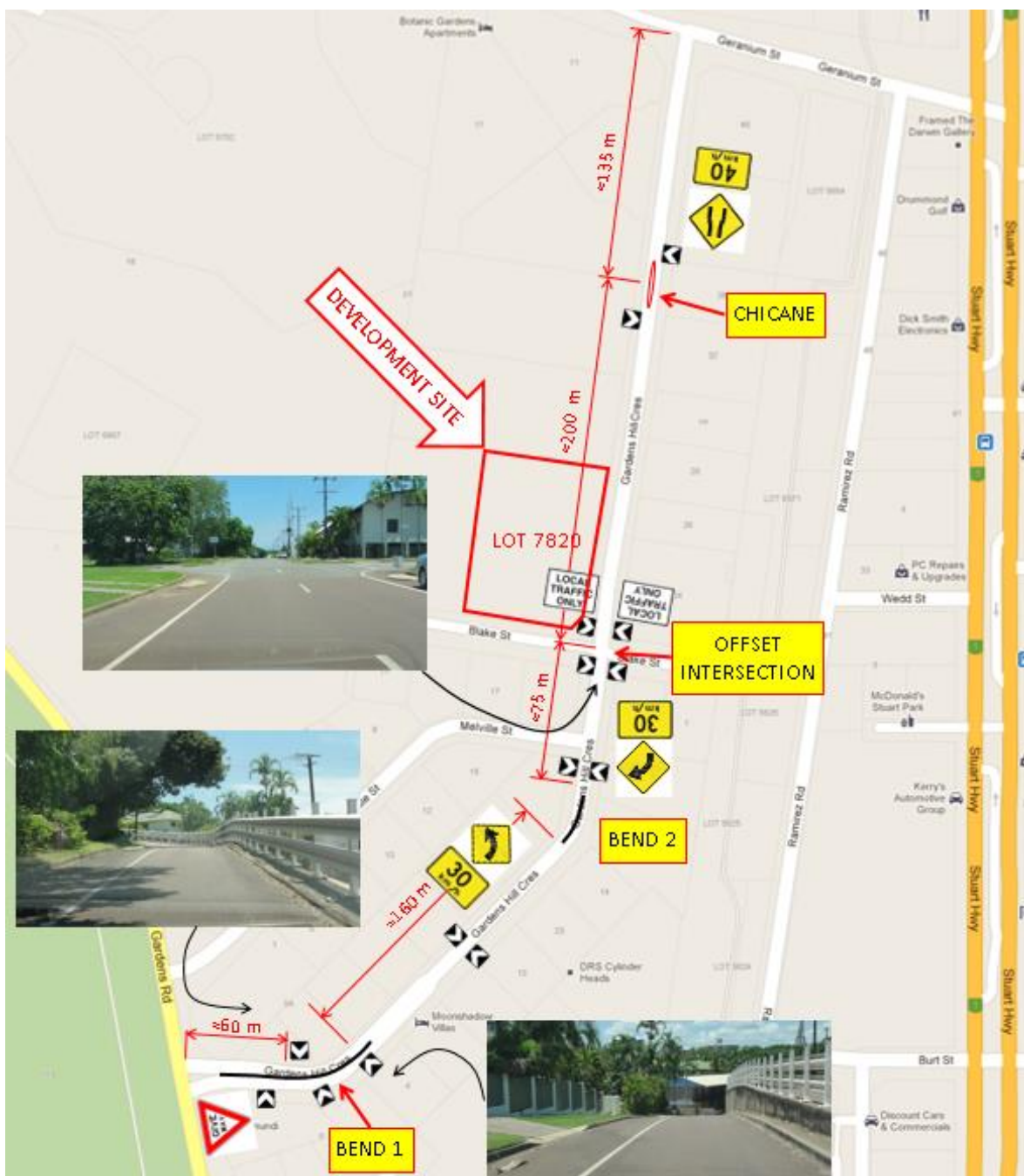
Figure 8 – Existing Local Area Traffic Management devices along Gardens Hill Crescent
