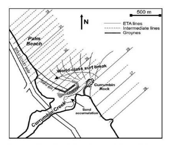
Fig. 2. Currumbin Creek and the southern part of Palm Beach in current configuration. Location of the groynes, the sand spit, the channel, the surfing break and the ETA lines.
