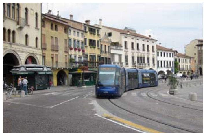
Innovative rubber tyre trams in Padua, with underground electric rail and battery power backup
