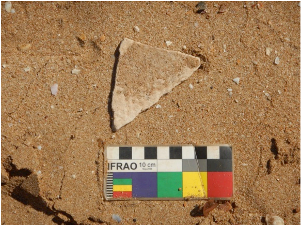
Figure 21. Asbestos on the beach.
