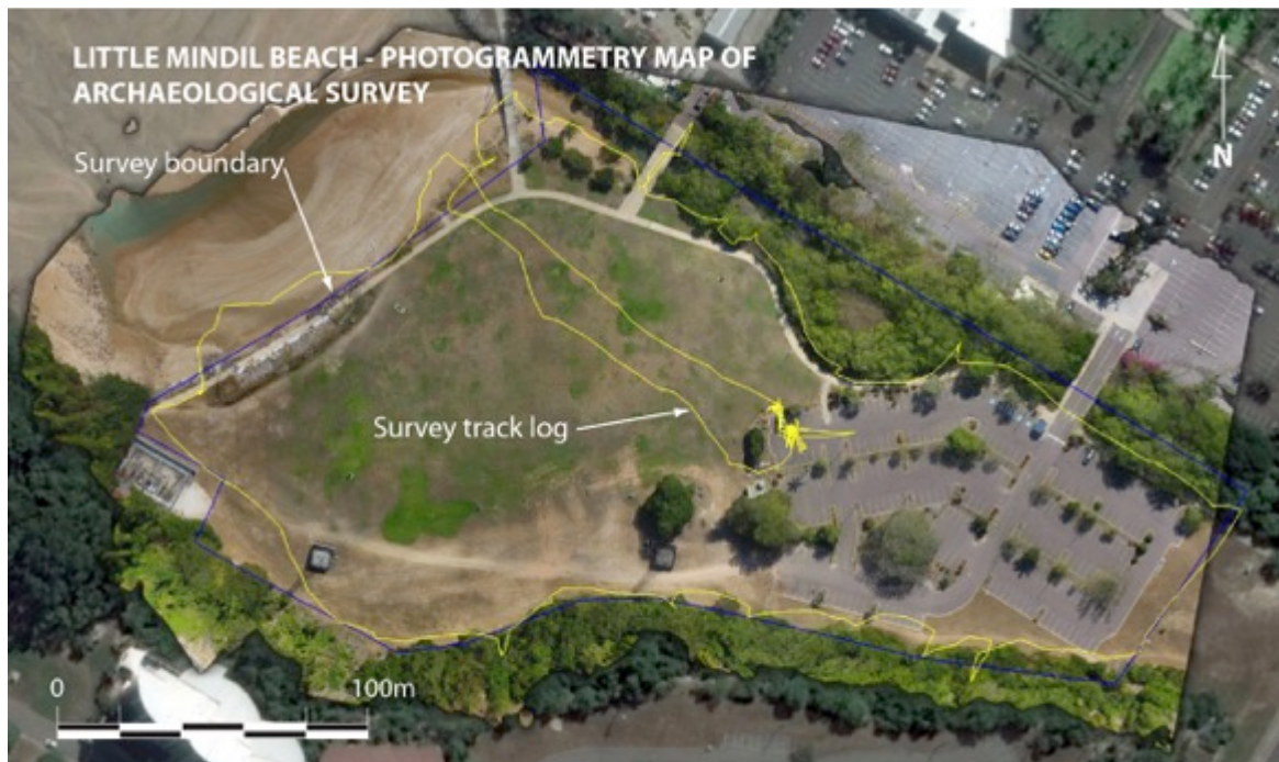
Figure 15. Photogrammetry survey of the proposed works area, superimposed with the survey track log.
